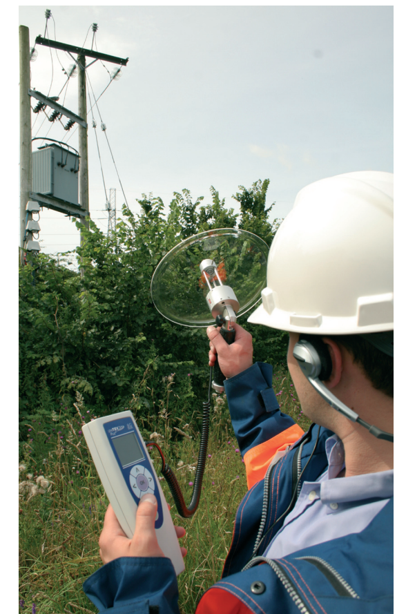
Listen for PD activity in overhead assets with the UltraDish™ add-on.
