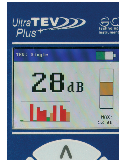
Menu-driven, multi-functional display of TEV and ultrasonic values.
